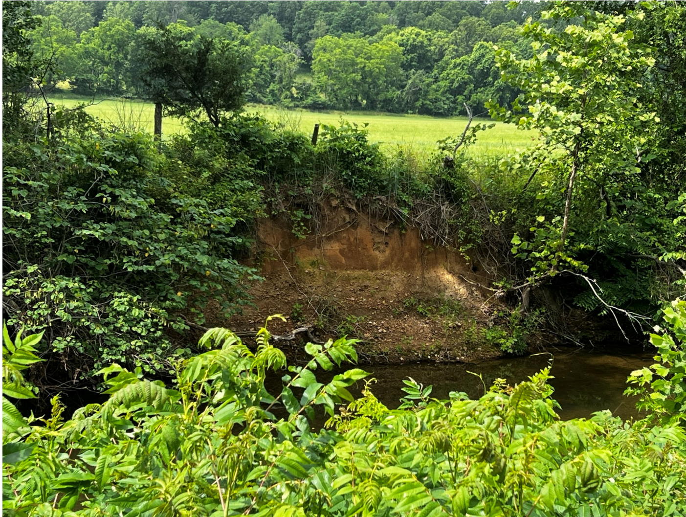
Alluvial deposits exposed in the north bank, west (downstream) of the existing bridge. These exposed deposits are typical of what was observed in the top 10-15 feet in borings (June 2023).
