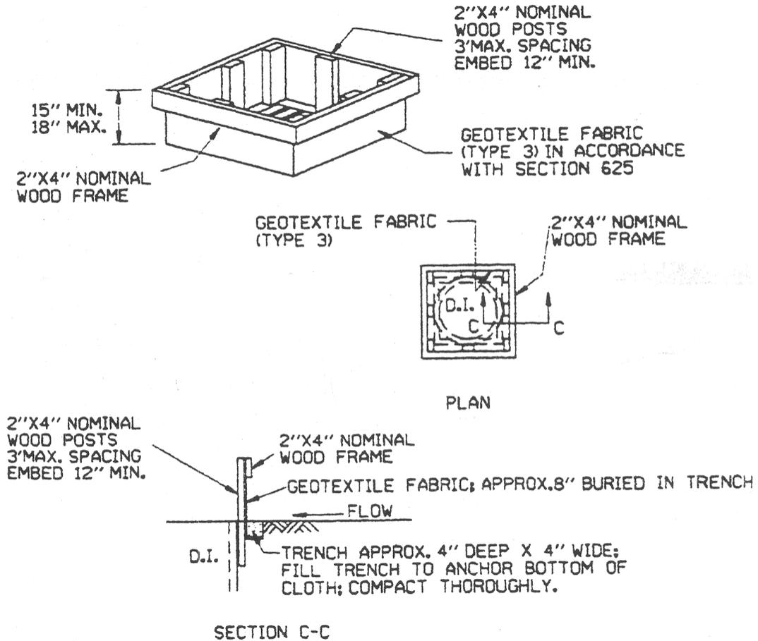
DROP INLET SILT FENCE
