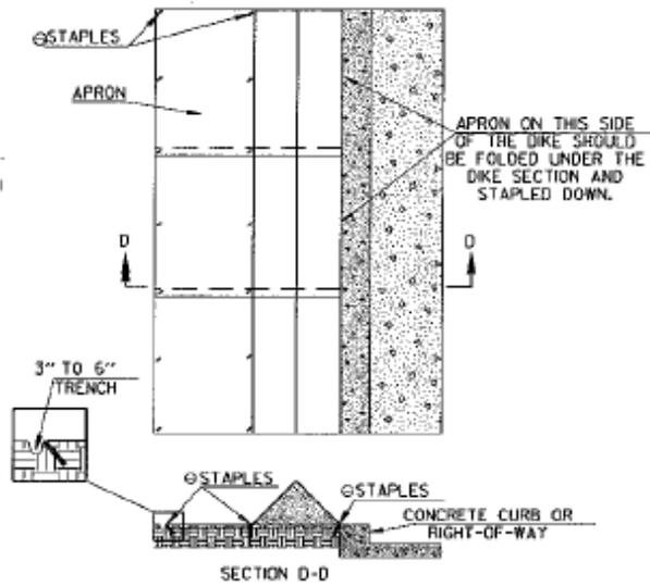
TRIANGULAR SILT DIKE INSTALLATION
