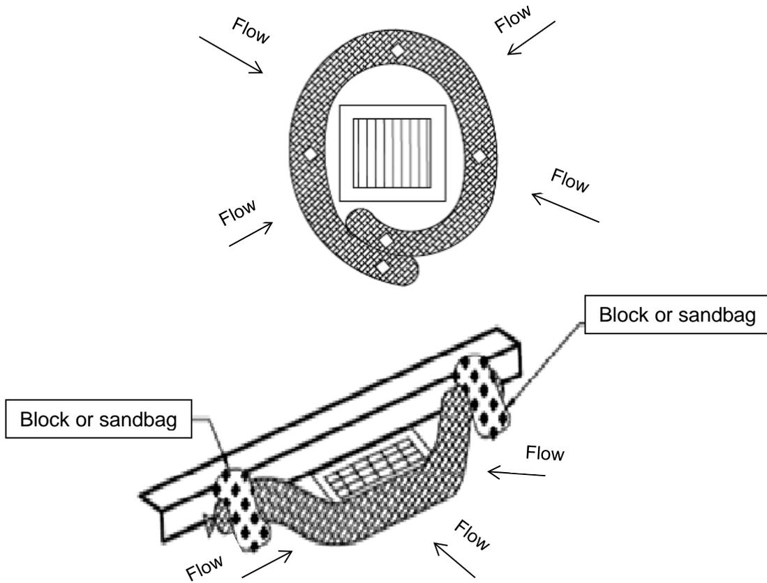
DROP INLET (top) and CURB INLET PROTECTION (bottom)
