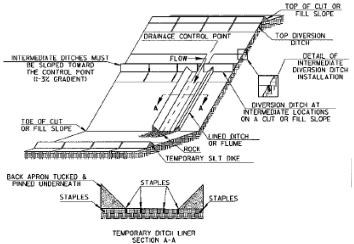
TRIANGULAR SILT DIKE INSTALLATION
