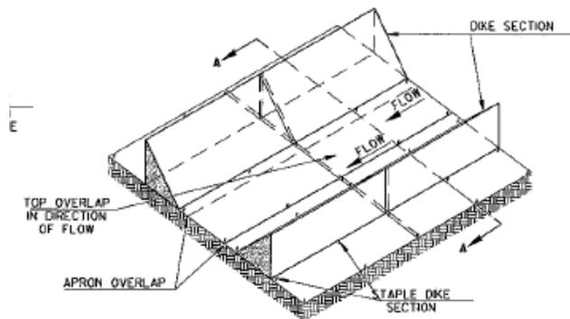
TRIANGULAR SILT DIKE INSTALLATION
