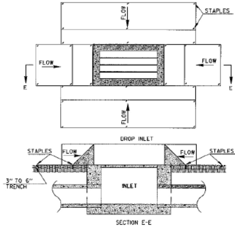
TRIANGULAR SILT DIKE INSTALLATION
