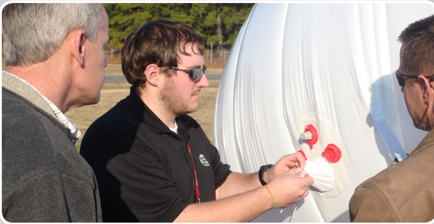
Daniel Siskowski prepares to deflate the balloon. The balloon can be deflated or inflated within approximately ten minutes.
