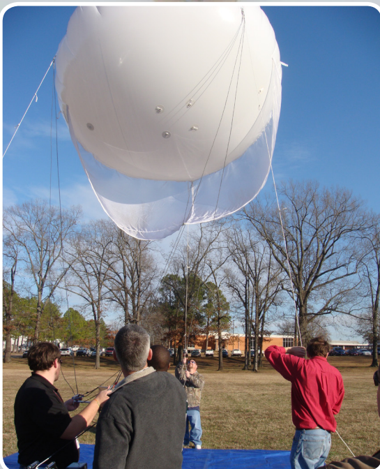
Filled with helium, the balloon is raised into the air and tethered to a winch on an AHTD truck.
