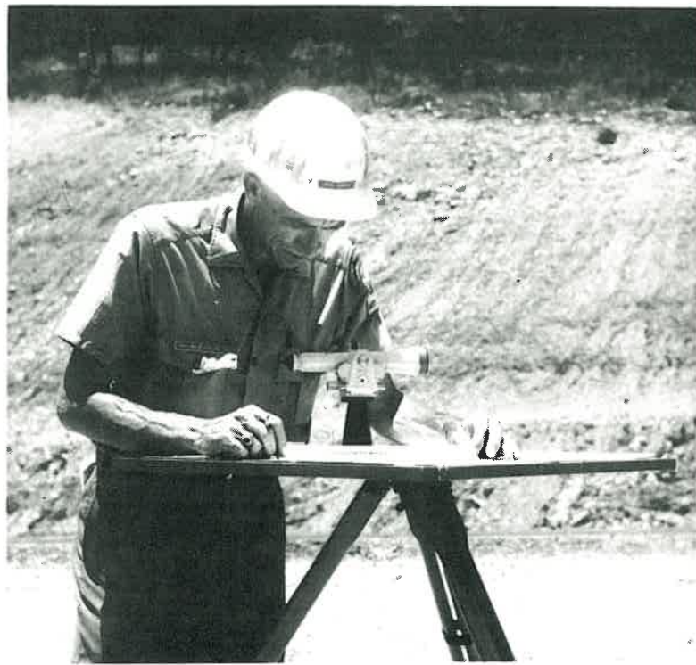
Bill Martin of the Forestry Commission takes a grade elevation for a scenic vista.
