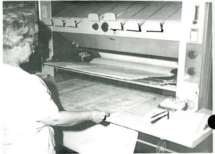
Lucille Huffstular is the operator of the Ozalid white print machine which has replaced the older model blue print machine. Blue or black ink is used to print on white paper.
