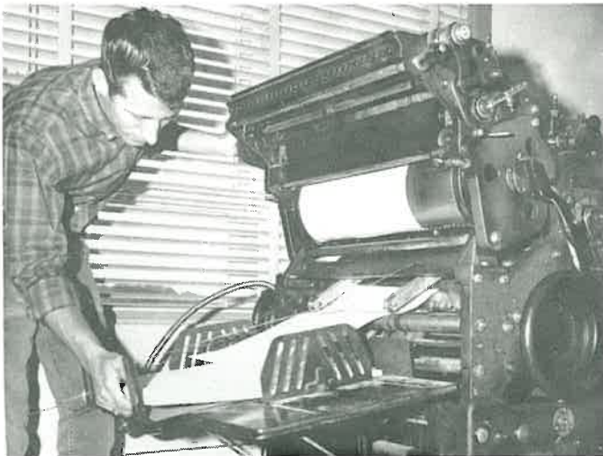
Guy Howard operates #266 offset press which can put out 5,000 prints per hour.
