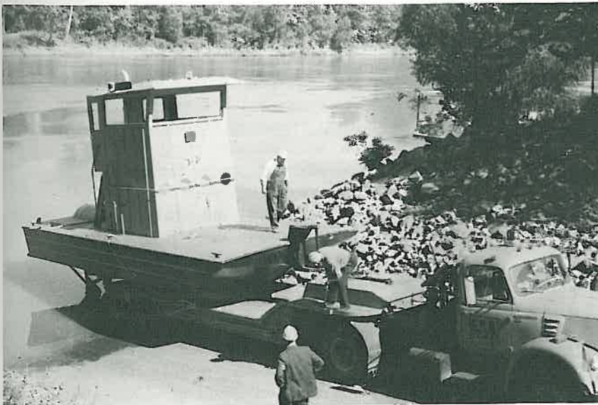
The tug is about ready to hit the water at St. Charles as workmen loosen security cables.
