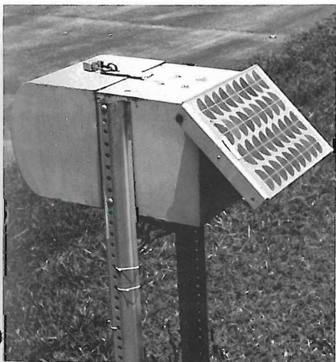
Solar panel attached to ATR provides a continuous source of electrical power.
