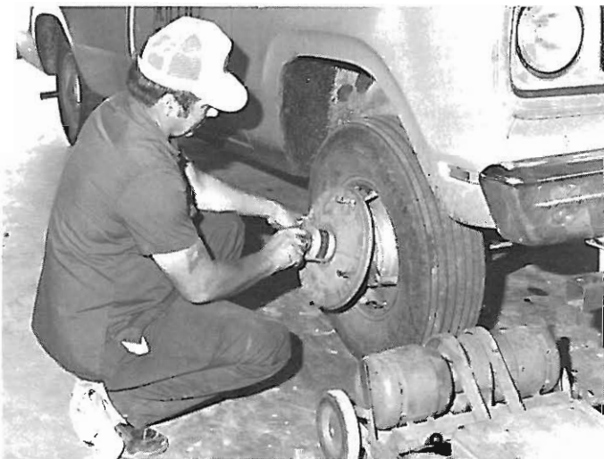
John Roy, a Senior Mechanic with 15 years service, balances wheels on a department vehicle at the District Headquarters.
