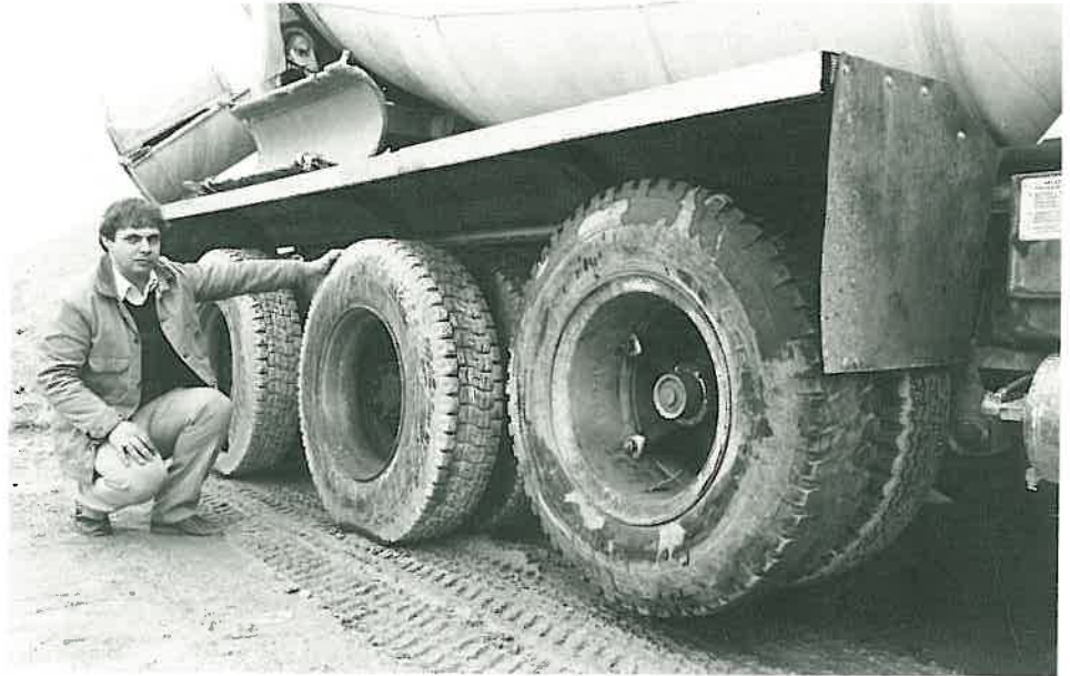
Dr. Thomas Parsons examines a truck with a "lift" axle, shown here in the raised position.
