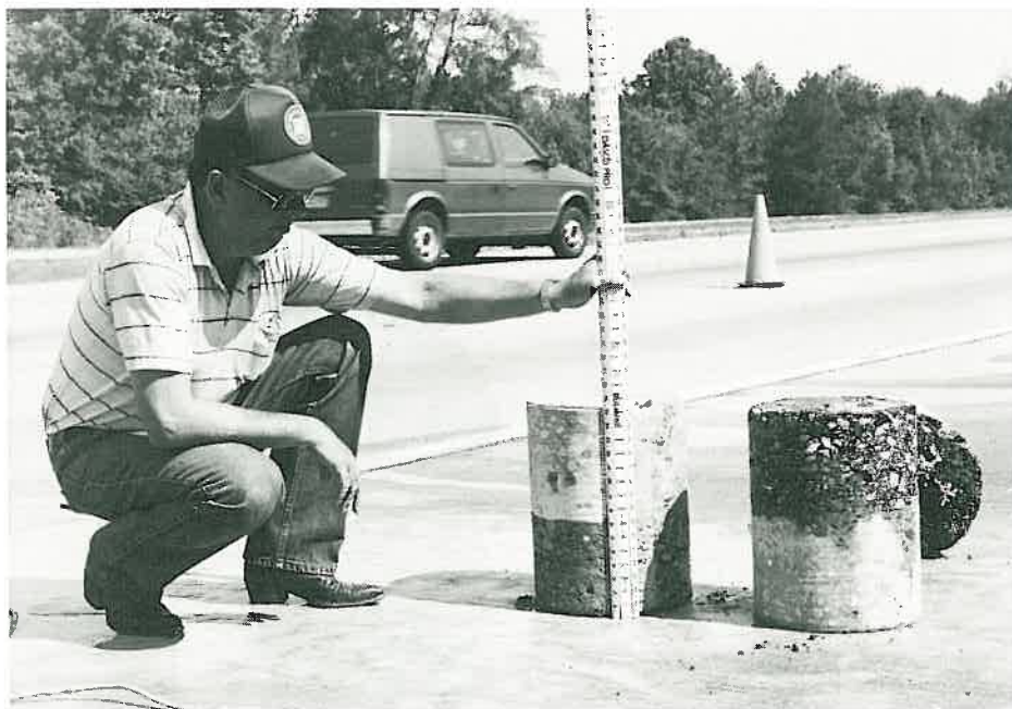
The core samples are measured for depth.
