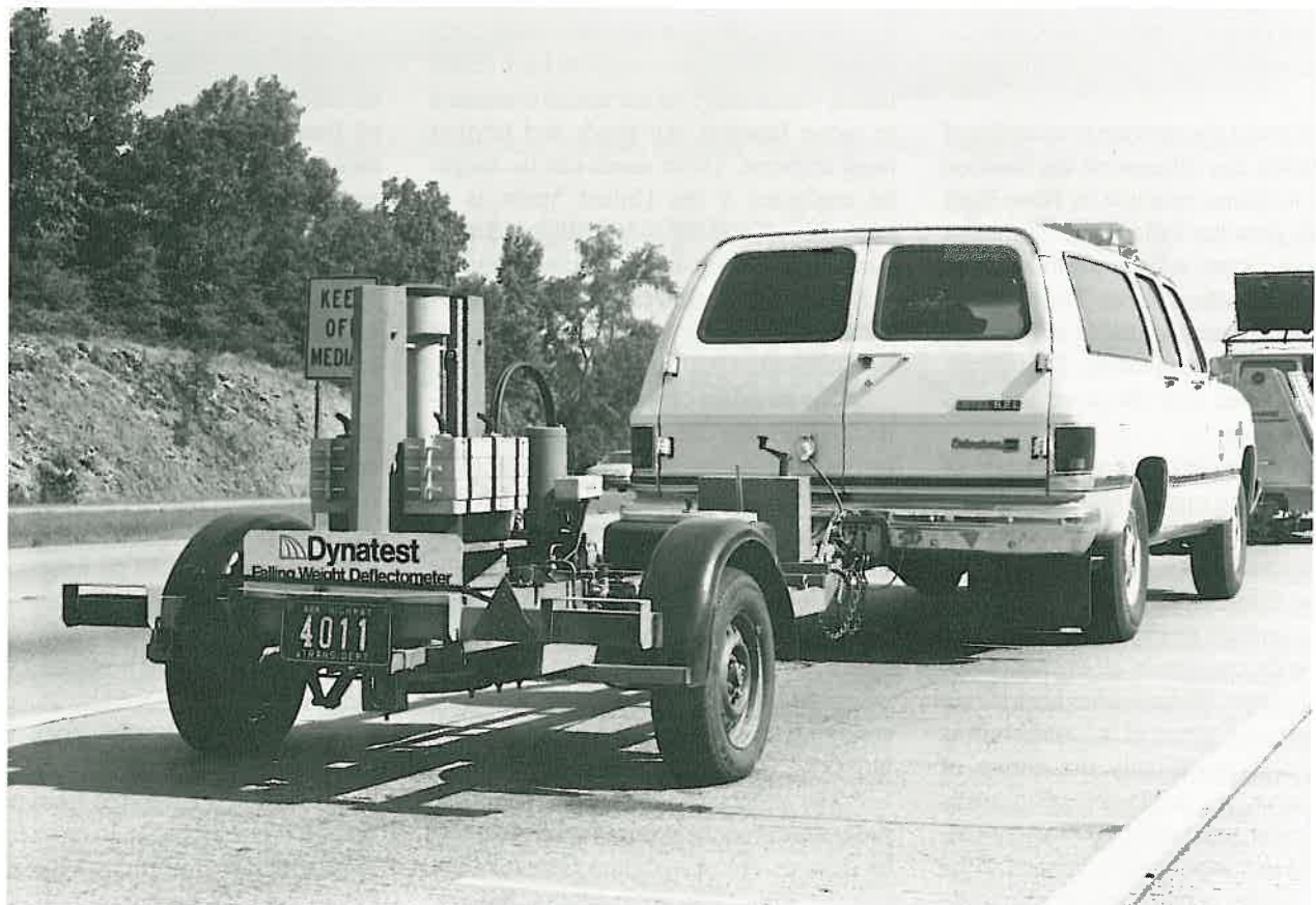
A Falling Weight Deflectometer measures the load carrying capacity of pavement.
