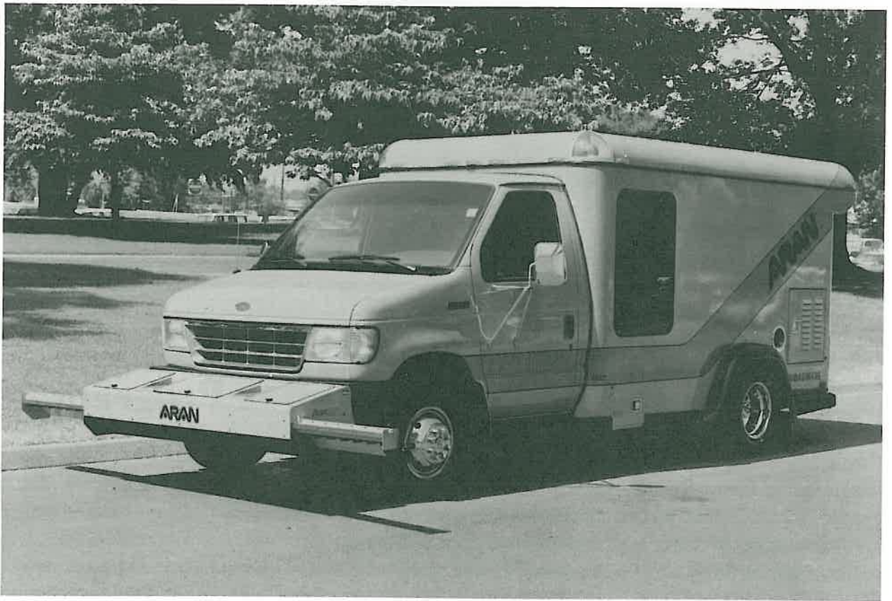
ARAN - The Automatic Road Analyzer Vehicle
