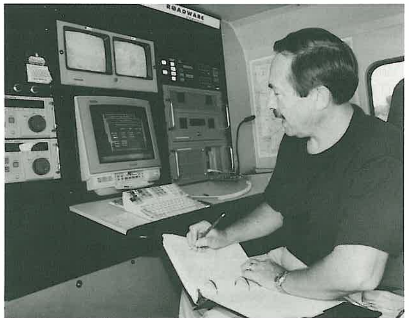
Gerald Stachurski , Highway Data Collector for the Programs and Contracts Division, operates the information-gathering equipment located inside the Automatic Road Analyzer (ARAN) vehicle.
