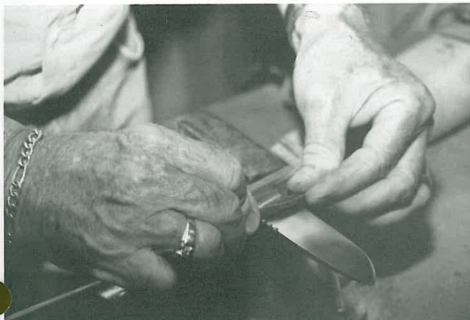
Polishing the blade using a round file and a small piece of fine sandpaper gives the knife a smooth, polished surface.
