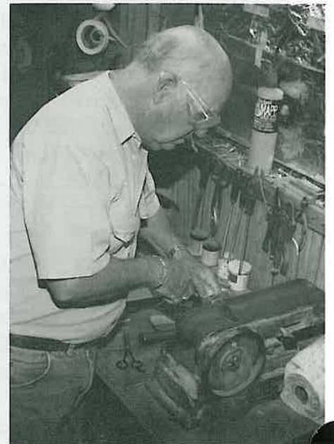
Sanding the blade down with a belt sander gives a rough finish before he proceeds with the final polishing.
