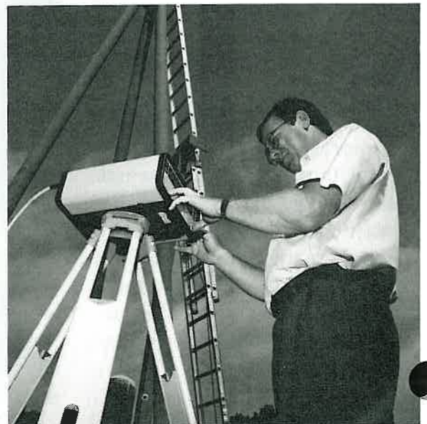
White adjusts a portable GPS receiving antenna.
