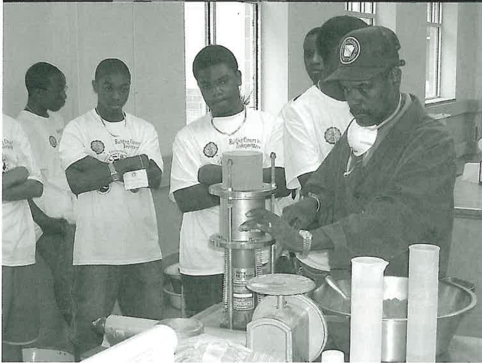
The students study Harold Banks, Materials Technician IV, as he uses a soil proctor to look for optimum moisture and maximum density of the soil.
