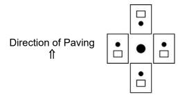
Calibration of the nuclear gauge using the direct transmission mode should follow procedures in this method but will require drilling four holes in the asphalt layer where the density is being taken at the positions indicated above.
