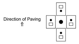
Calibration of the nuclear gauge using the direct transmission mode should follow procedures in this method but will require drilling four holes in the asphalt layer where the density is being taken at the positions indicated above.
