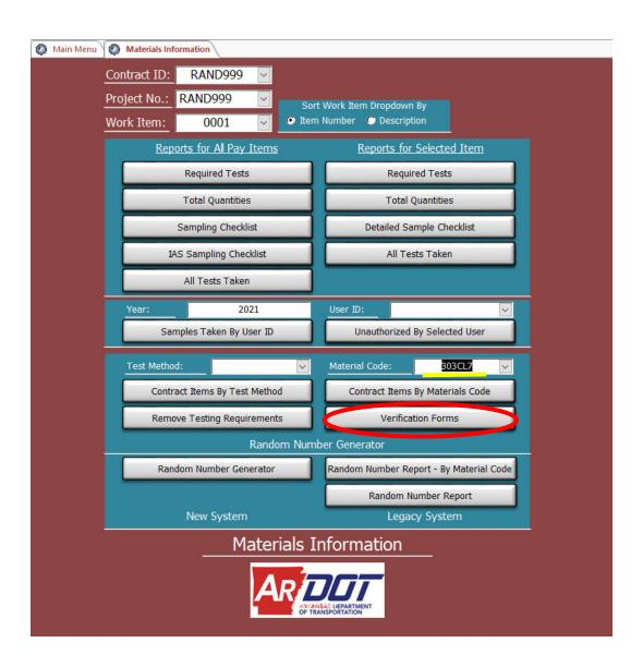
Fill in the information by selecting Sample IDs in the drop down menus. Once the Contractor Test and the ARDOT test has been filled in select "verify test". It will indicate if a test met the verification requirements for material.
